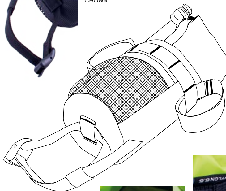
STRAP WITH CAMLOK BUCKLE TO FIX THE BOTTOM OF THE FORK CROWN.
