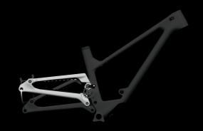
A suspension system with a high pivot point that results in a rearward axle path throughout its travel.
