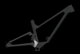
Our Rate Control Linkage is used to manipulate the leverage rate as the suspension compresses.
